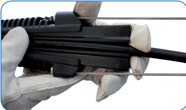
Push on the wedges by hand to initiate the gripping onto the cable
